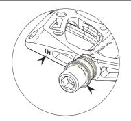
Identify right hand and left hand pedals by looking for the groove on the LH pedal spindle shoulder or the LH mark on the pedal body.
